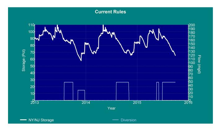
The plot below shows the overall improvement in reliability by virtue of the current, forecast-based rules. The drought exercise indicated a greater desire by operators to pump more water in the summer months to preserve storage during the drought season and a preference to pump less water in the winter months when the cost of pumping relative to water sales is higher.
